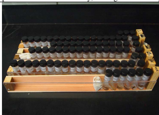
Fig. 4. Final product: specimens and labels moved to 4 dram glass vials with polypropylene beveled insert in screw cap.
